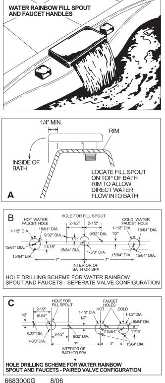
Using a scribe tool or awl, mark the center points for all holes, then remove the template.
